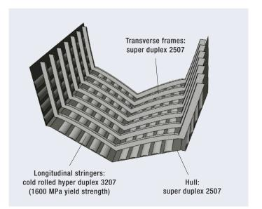
The stringers are spot welded to the hull plates. The frames, welded to the stringers, are not in direct contact with the hull. The flexibility of the stringers allows them to absorb the wave force preventing the hull from bucking.
