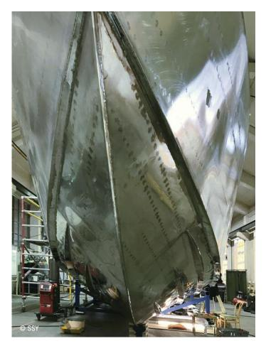
Stainless steel hull of a prototype at the ship yard before mirror-polishing under the waterline and painting above it.
