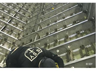
> Welding of the interior structure of a ship.
